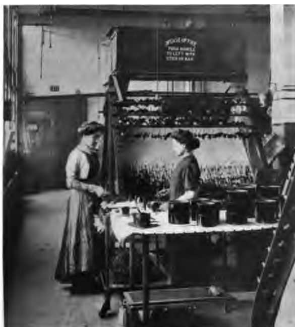
Fig. 5. Sand Box to Extinguish Fire in Japping Outfit, etc.†
